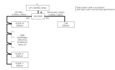
\* Encoder Input Wiring: See Installation Instruction II097
