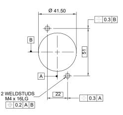
Details shown above are for vertical fixing, for horizontal fixing, details are rotated 90 degrees.
