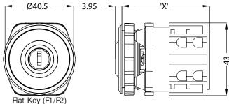
M-20 key switches can be supplied lose or incorporated into stations with 1.0mm to 2.5mm stainless steel faceplates. Recommended mounting pitch vertically & horizontally is 50mm. M-20 key switches can accommodate faceplate thicknesses from 1.0 mm to 3.0 mm.
